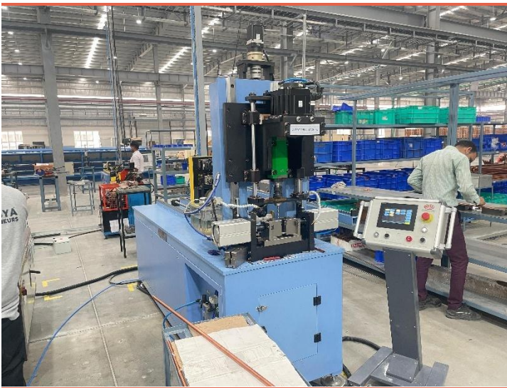
Exhibit 16: Tube forming machine in header section
