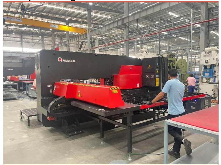
Exhibit 17: Turret punch press machine for sheet metal processing
