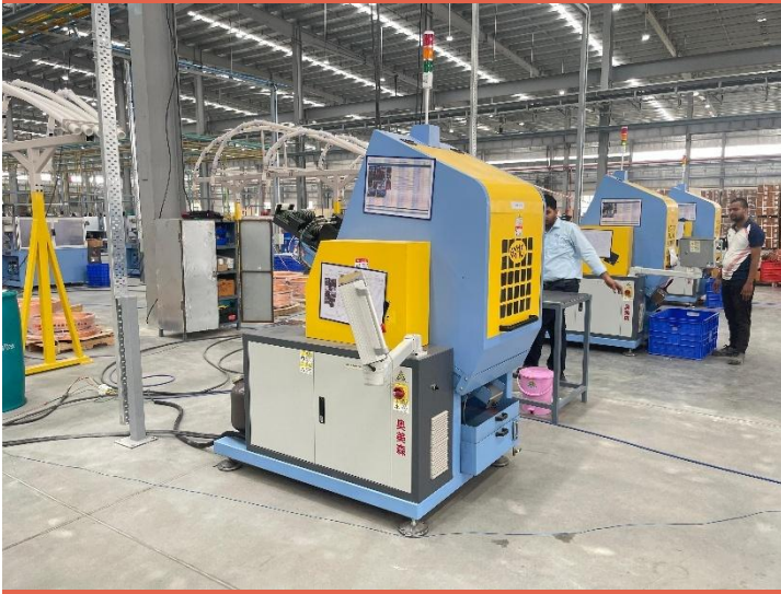
Exhibit 14: U bend processing machine
